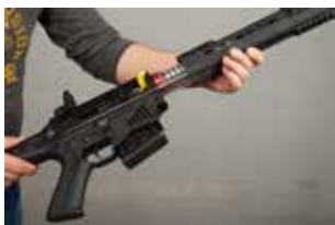
Photo 12-) You can pull easily forend of AR12 as in the photo, if you operated the process in Photo 11.
