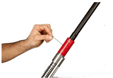
Photo 13-) Unscrew the fixing screws which are on the gas cylinder with 2,5mm allen wrench which are sent you in box
