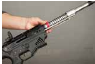
Photo 15-) You can disassemble bolt group of AR12 completely after required steps as in the photo easily.
