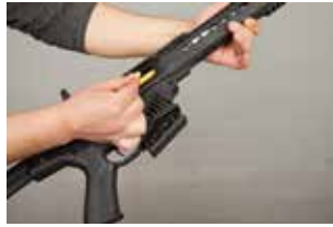
Photo 2-) Pull AR 12 charging handle to operation direction then use shell safety kit (yellow part) to make ready your gun disassembling in right way. If you do not use that shell safety kit, you will damage shell carrier ramp absolutely!!!
