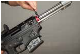
Photo 14-) Use your AR12 Special Wrench Set for turning the barrel nut of your gun.
