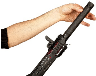
Photo 4 -) Turn AR12 muzzle break by using your hand to direction of clockwise until thread on barrel allows to disassemble muzzle completely.
